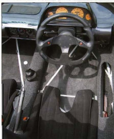
The cockpit is just the way it should be – simple and effective. Note colour-coded guagery, cutaways in seat bases to provide stepping point, side storage pods and exposed cross-bracing.
