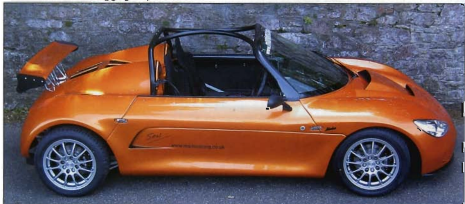
Curved rollcage top tubes make access easier and add to curved lines.
